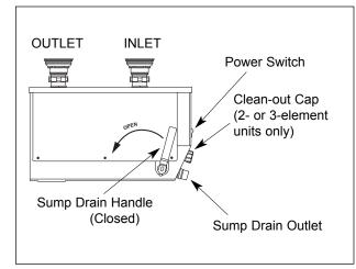
Figure 8. Hydro-Heater Side View
